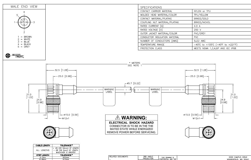
8-29mm ±1.0mm 30-49mm ±2.0mm 5<u>0</u>-69mm ±3.0mm 70-100mm ±4.0mm OVER 100mm ±5.0mm \* UNLESS OTHERWISE SPECIFIED
